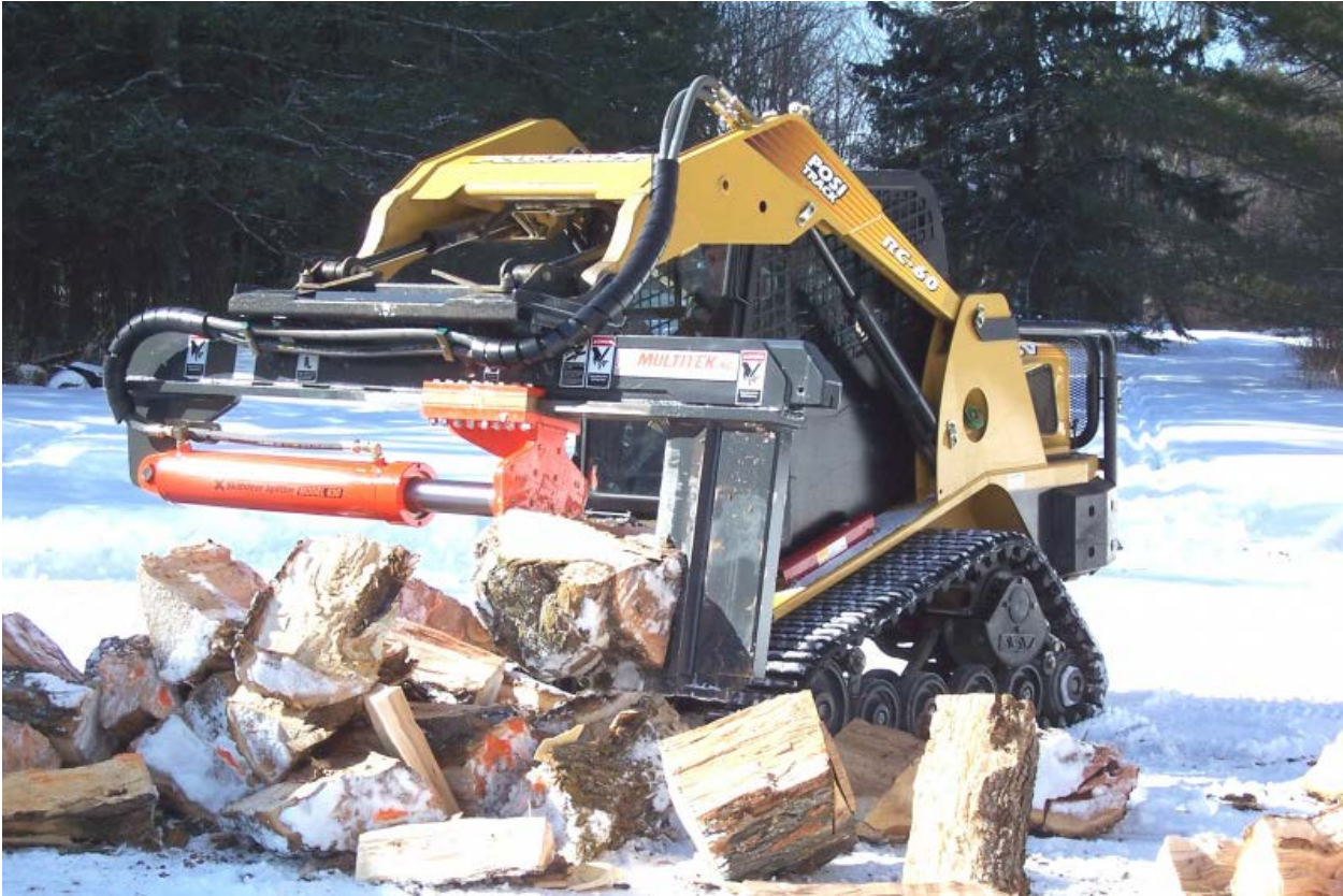
Log Splitter Attachment (shown as an attachment on a track skidsteer loader)
